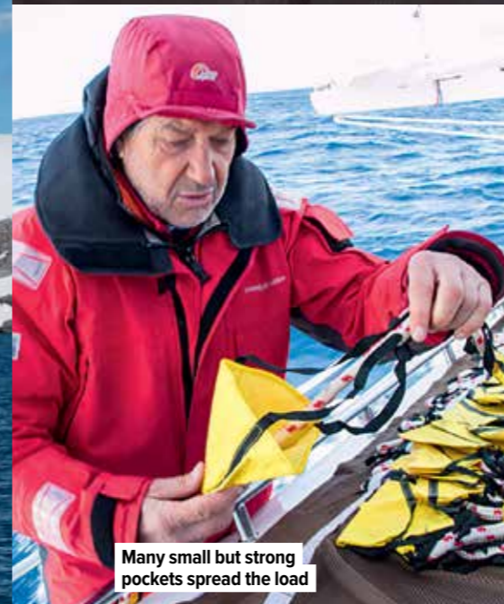
Each JSD is custom made, the length and number of pockets proportionate to the size and tonnage of the yacht
